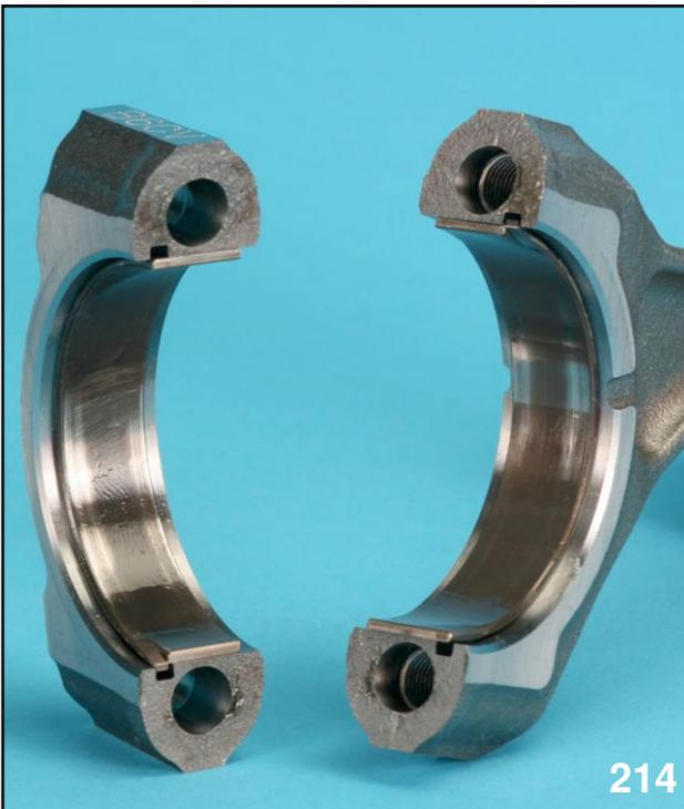
CONNECTING ROD CAP SEPARATED FROM ROD
