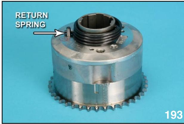
EXHAUST CAMSHAFT SPROCKET AND RETURN SPRING
