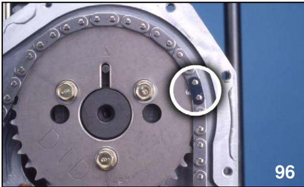
*LEFT BANK INTAKE CAMSHAFT TIMING MARK*
